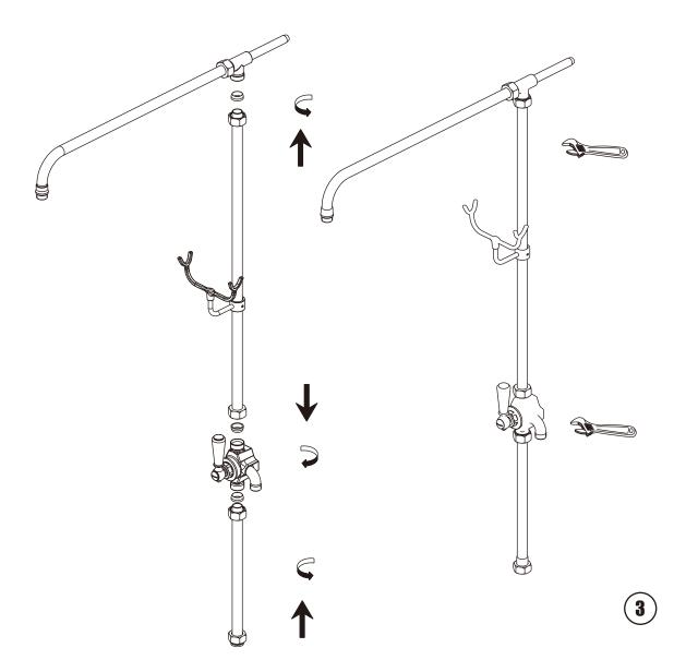
Put the compression olive into the riser bracket and then fix the riser with the bracket. Put the compression olive into the diverter body and then fix the riser with the diverter body. Tighten the nut by wrench in order to fix the riser with the bracket and with the diverter body.
