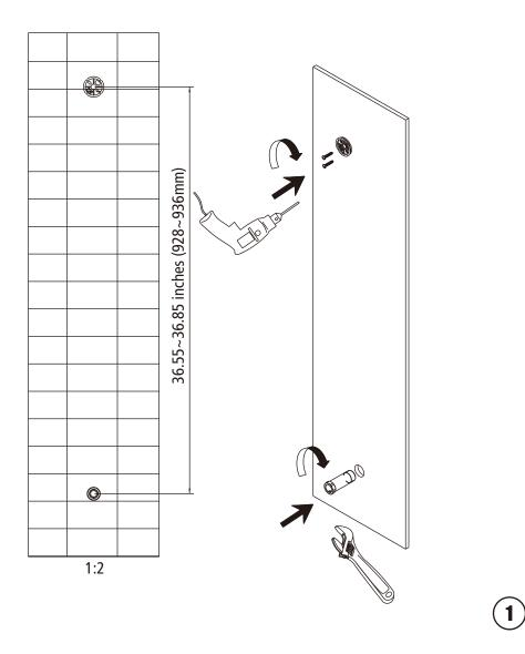
Install the Inlet and locate the wall bracket. Make sure that the distance between the inlet and the wall bracket is 36.55~36.85 inches (928~936mm).
