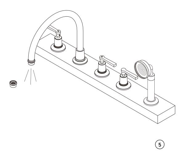
**5** After installing faucet, remove aerator and open the hot and cold supplies. Check for leaks.
