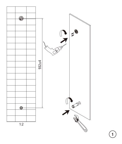
1 Install the Inlet and locate the wall bracket. Make sure that the distance between the inlet and the wall bracket is 36.55~36.85 inches (928~936mm).
