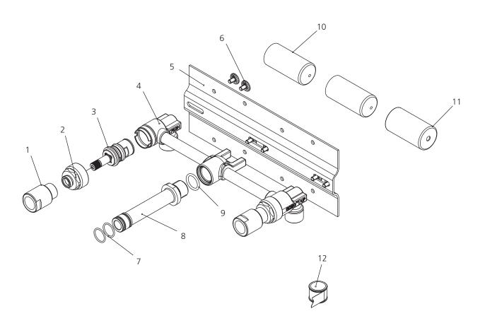
Adaptor (067186) O-ring (048096N) 7 2 Retaining nut (016231) 8 Adaptor (039958) 3 Cartridge (507909N) 9 O-ring (004010N) Body (061058) 4 10 Protective cap (038007) Protective cap (045433) 5 Back plate (126671-S) 11 Screw (008013) Teflon tape (203000) 12
